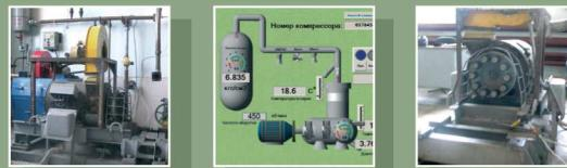
The stand is designed for the automated testing of the compressors of any type
