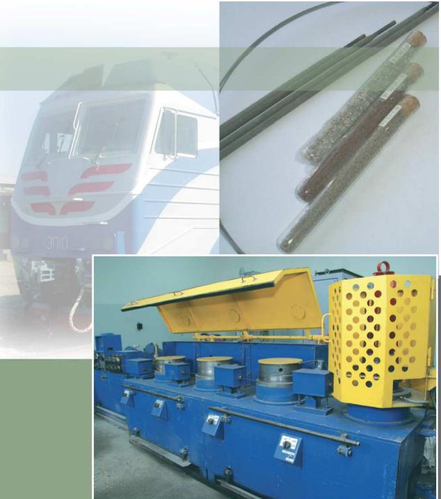
The flux -cored electrode is designed for welding and facing the structures made from low-carbon and low-alloyed steels
