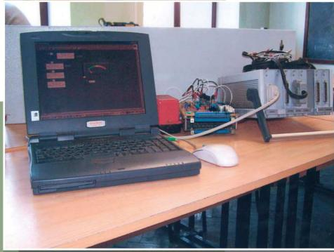
The system is designed for diagnosing the control electric circuits of machine VPR - 02, adjustment of testing instruments (gages)
