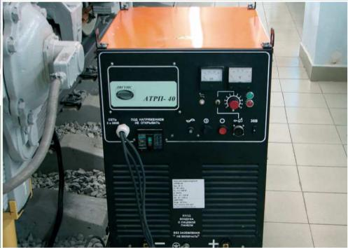
*The unit contains a thyristor converter and power circuits for the traction electric motor power supply*
