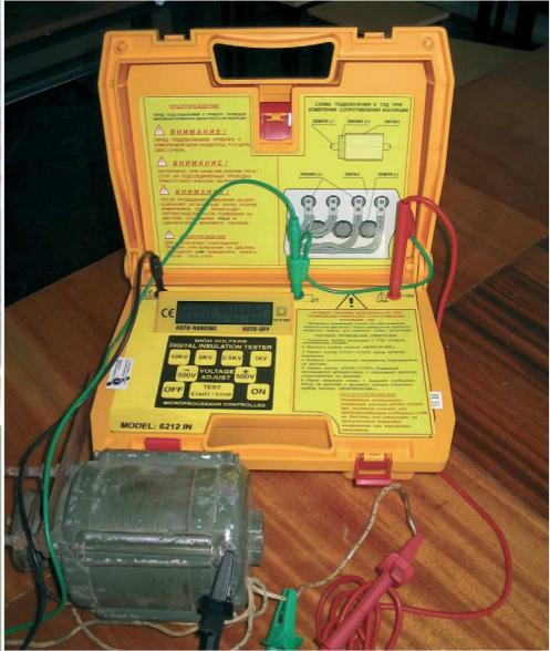
The diagnostic system is intended for defining the condition of isolation of an electric equipment of electric locomotives with an alternating current during the scheduled repairs in locomotive depots
