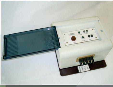
*The device is intended for the control and measurement of the isolation level of power circuits of an electric locomotive of an alternating current*
