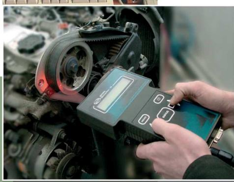
Purpose Diagnostics of a technical condition of diesel engines fuel equipment
