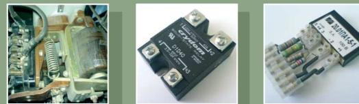
**The contactless relay made on the basis of semi-conductor elements, allows to replace standard electromechanical relays of circuit control of an electric locomotive.**
