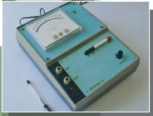
*The device is intended for the detection without disassembly of short-circuited coils of any winding of the electric machine having separate outlets, including transformers*
