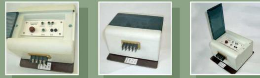
**The device is intended for the control and measurement of the isolation level of power circuits of an electric locomotive of an alternating current.**
