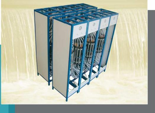
The installations "Akvakhlor" is designed for sterilization and water reclamation
