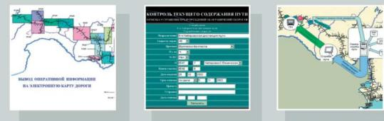
This technology is intended for organizing the dispatch control of the device status condition of track facilities on the road through CDS (Communication Data System) with transferring the data about the technical device status condition and their abrupton from the roadway enterprises and the computerized troubleshooters to the server of the railroad computer center (IVTs).
