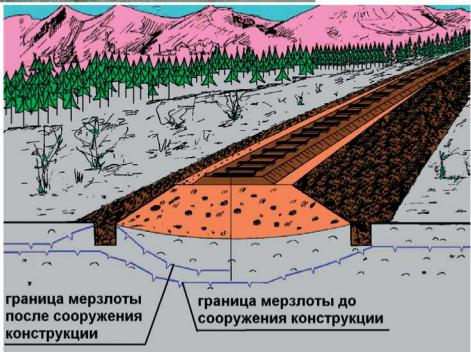
The construction is used for the stabilization of the road and pipeline mounds on the weak bases
