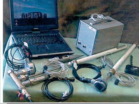
*It is intended for diagnosing the conditions of the grounds of road-beds and bases under the influence of vibro-dynamic loads on the objects under examination*
